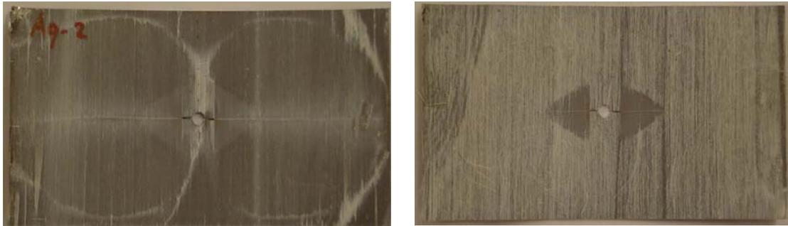
Figure 5: Large delamination on outer metal/S2-glass prepreg interface (left) and normal delamination in second metal/S2-glass prepreg interface (right).
